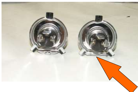
4: You must trim bottom flange of bulb to allow clearance for the LED wires to exist the housing.
