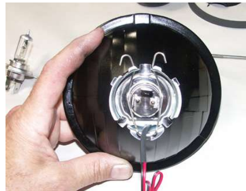
5: Re-install the bulb into the housing. Be careful not to pinch the new LED wires.
