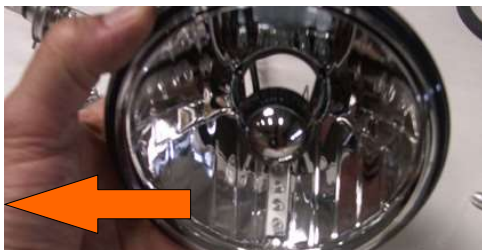
3: Slip LED through hole and into the bottom of the housing. Align and press in place.
