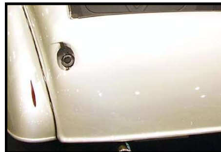
6. Weld in fuel door. Seam seal all the seams, then finish body and paint work.
