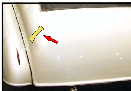
2. Use the template to find the best position for the fuel door.
