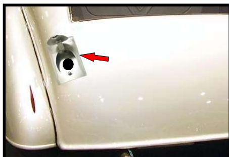
4. Slip assembly in the cut out. Mark and enlarge the hole to fit.
