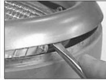
When installing or removing the trim it is best to put a few layers of masking tape on the painted surface so you do not scratch the paint.
